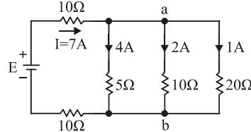
$V_{ab} = 2 \times 10 = 20$  V,  $I = \frac{20}{5} + 2 + \frac{20}{20} = 7$  A
