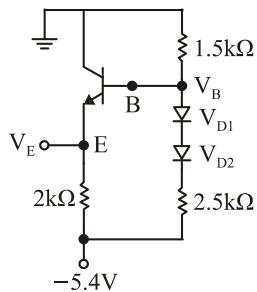
$$V_B = (-5.4 + 1.4) \times \frac{1.5 \text{ k}}{1.5 \text{ k} + 2.5 \text{ k}} = -1.5 \text{ (V)}$$
