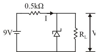
$$\begin{aligned} \text{考慮 Zener 內阻} \Rightarrow V &= V_{ZK} + r_Z \times I_{ZK} \\ &= 6.7 + 20 \times 0.2 \text{ (mA)} = 6.704 \end{aligned}$$
